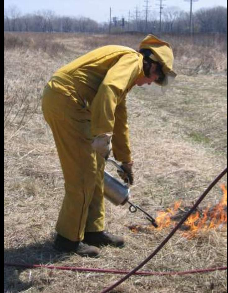
Drip Torch to Ignite. A mixture of diesel (~70%) and gasoline (~30%).
